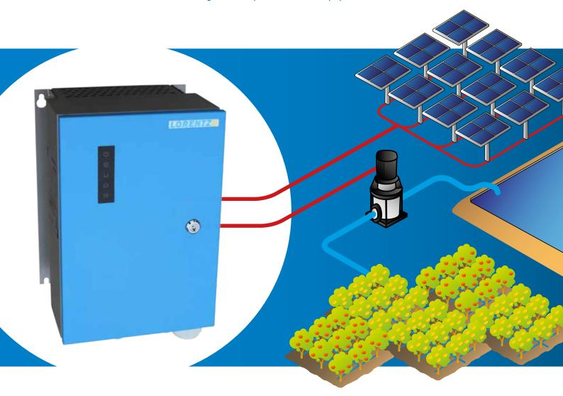
PSk2 is an integrated solar water pumping system for larger applications.
